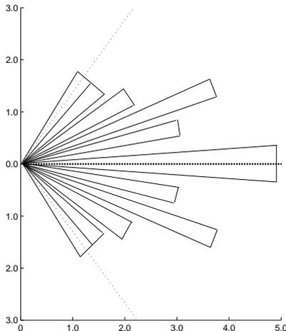
**Figure 2: Horizontal detection area  $[m^2]$  according to the PIR data sheet.**
