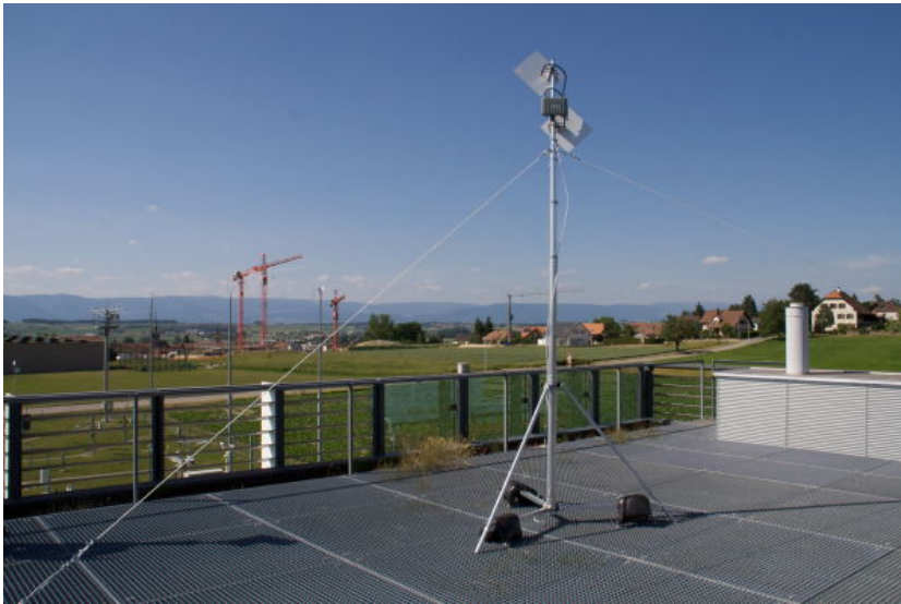
Figure 5: Node06 mounted on the platform roof of the MeteoSwiss building in Payerne.
