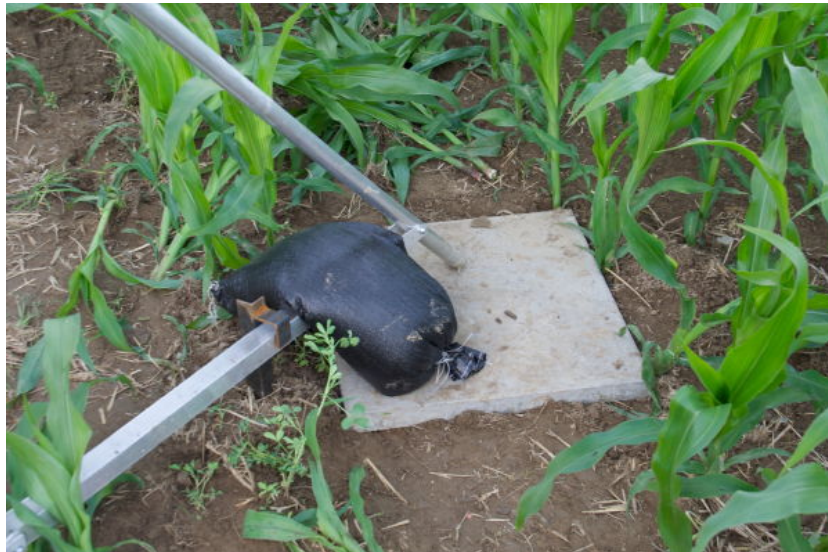
Figure 10: Concrete paving slab to prevent sinking in of the tripod, sand bag and iron stake to stabilize mast.
