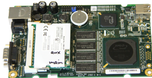
Figure 6: Mesh node: PC Engines Alix.3D board with two IEEE 802.11a/b/g/h miniPCI cards and a battery for the real-time clock.
