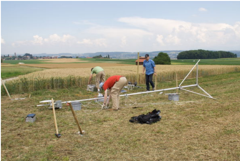
Figure 9: Complete assembly of telescopic mast in horizontal position before final setup.
