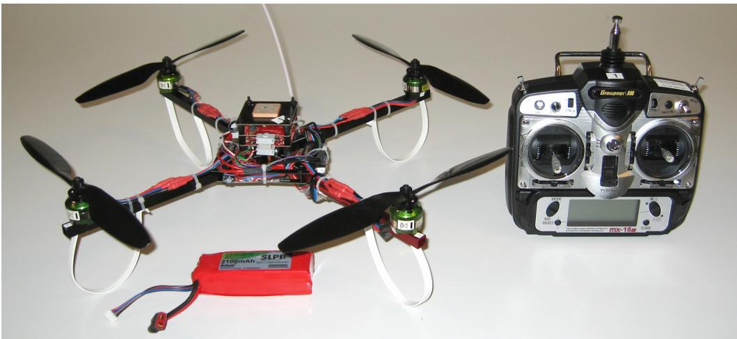
**Figure 2.2:** Assembled Mikrokopter kit.
