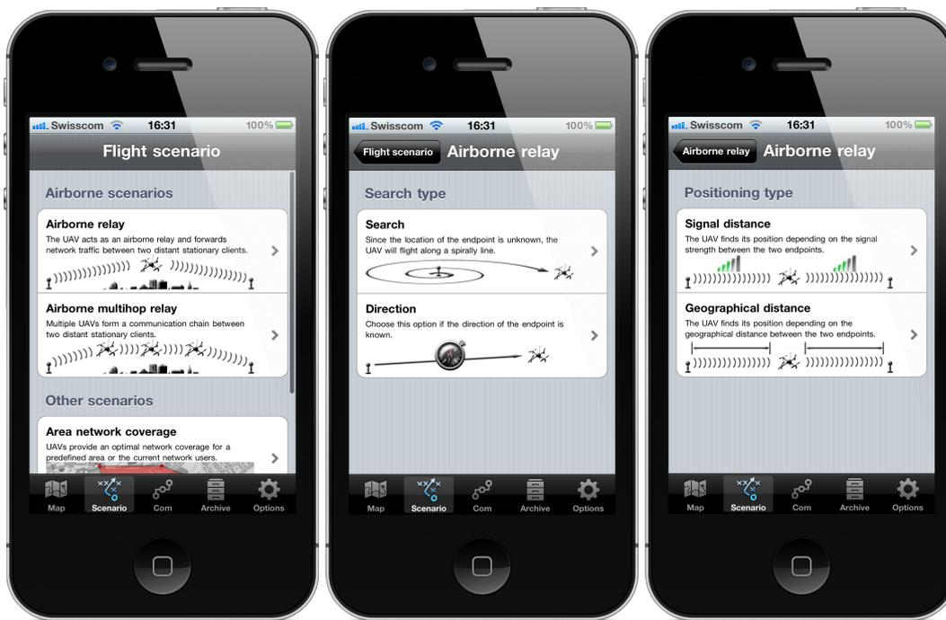
**Figure 2.8:** *Remote Control App* on an iPhone: Selection of the deployment scenario [31].
