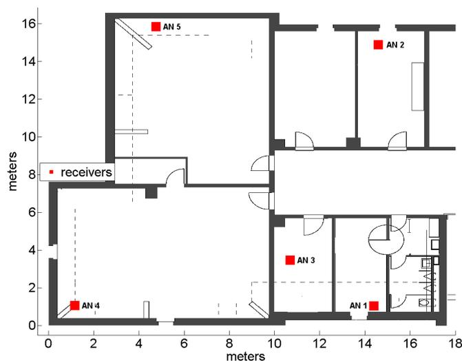
The Anchor Nodes (ANs) were deployed on the third floor of IAM building at University of Bern. Figure 4.1 shows the floor plan and the deployed ANs.
