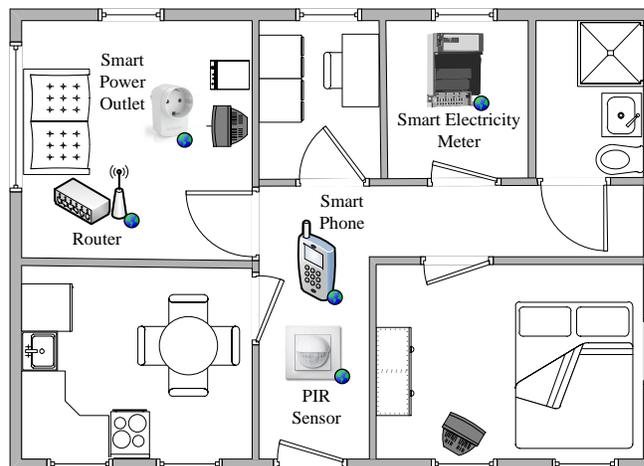
Figure 1. A possible opportunistic sensing scenario with a smart phone, a wireless router, a smart power outlet, a smart meter and an infrared (PIR) sensor.
