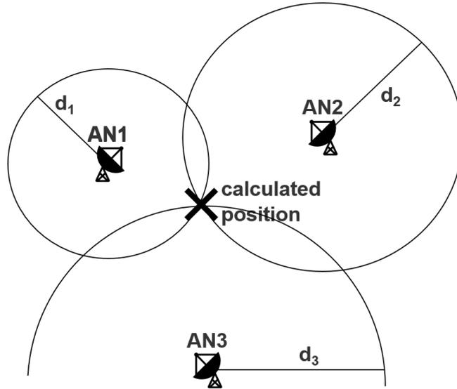
FIGURE 2.3: Graphical illustration of the trilateration concept.
