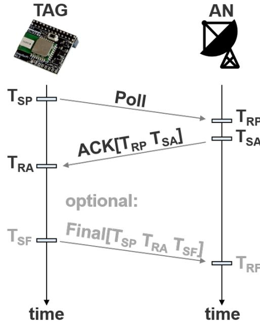
FIGURE 2.1: Illustration of TWR and SDS-TWR communication
