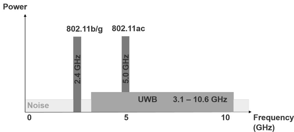
FIGURE 2.4: Comparison of Wi-Fi (802.11) and UWB frequencies.
