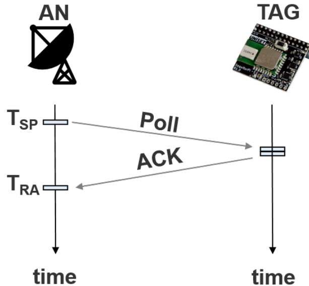
FIGURE 4.1: Minimal implementation of Two Way Ranging.
