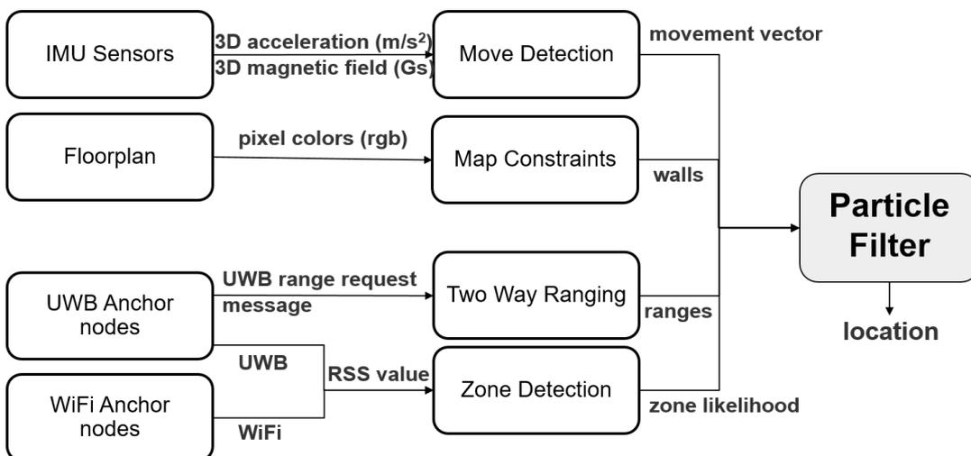
FIGURE 3.2: Overview of the localization algorithm components.
