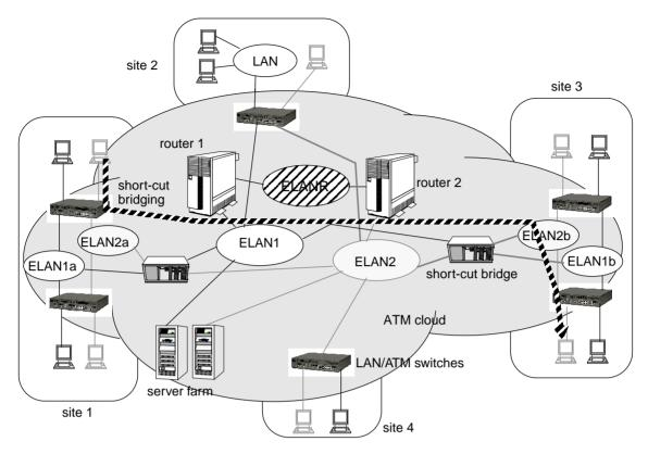
Figure 3: VLAN architecture with short-cut bridging
