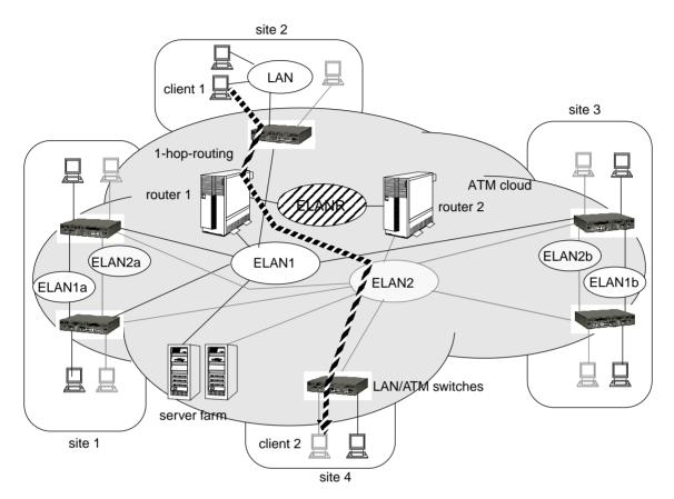
Figure 2: VLAN architecture
