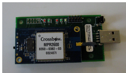
Figure 11. MRP2600 MicaZ node connected to the USB board
