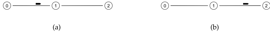
Figure 4.2: Nam output for the script listed above. (More information about Nam is provided in section 4.6.2.) The UDP protocol Agent on Node 0 sends a packet addressed to one of the Agents on Node 2. This packet is forwarded by the Node and Link components to the receiver, which discards it.
